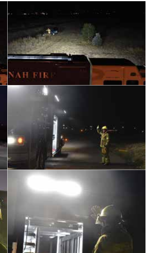
PERIMETER LIGHTS 1 WHELEN M9 AND 2 FIRETECH FT-B-45 (46" LED STICKS) ON EACH SIDE OF THE TRUCK
