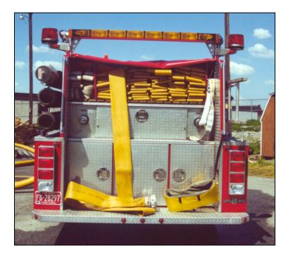
Figure 16: Arrow bar mounted high on the rear of a fire apparatus. *Photo credit: Jack Sullivan.*
