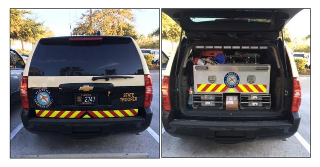
Figure 9: Florida Highway Patrol SUV with conspicuity markings inside and outside the liftgate. *Photo credit: Florida Highway Patrol.*
