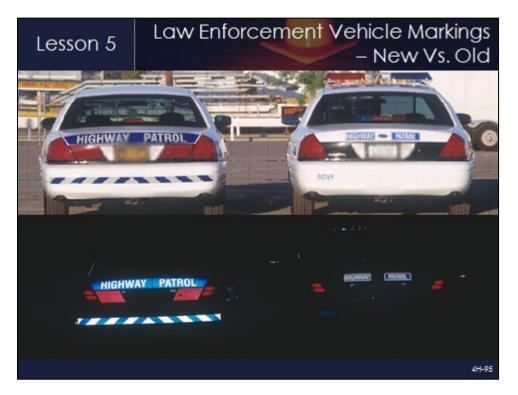
Figure 1. Comparison of conspicuity of "new" vs. "old" retroreflective vehicle markings on the rear of Arizona Highway Patrol cruisers. Image from the National TIM Training Program (Rev 7/13). *Photo Credit: Federal Highway Administration.*
