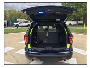
Figure 4: Retroreflective tape inside emergency vehicle doors and liftgate. *Photo credit: Massachusetts State Police.*
