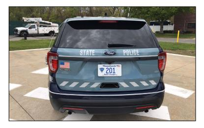
Figure 5: White retroreflective material in a chevron pattern on the rear of an MSP vehicle. *Photo credit: Massachusetts* State Police.
