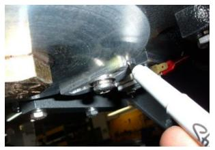
With the centering cam slightly loose, it may be easier to adjust its position by tapping on its edge with the assistance of a socket driver rather than attempting to move by hand.
