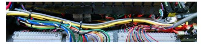
Wire the 10 Awg blue/white and green wires to the middle pole strip in the relaybox. Also wire the smaller cable into the middle pole strip in the relaybox.
