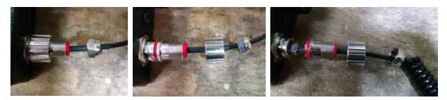
Make sure the tab on the ethernet (CAT 5) connector is in the slot before attaching the cord. Lock the large nut, make sure the ethernet cord is pushed all the way in, lastly tighten the small nut onto the cord.
