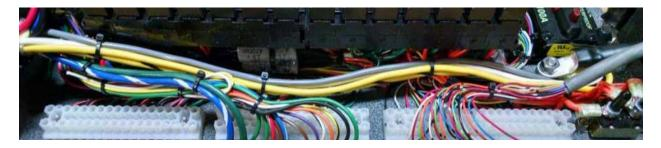
Wire the 10 Awg blue/white and green wires to the middle pole strip in the relaybox. Also wire the smaller cable into the middle pole strip in the relaybox.
