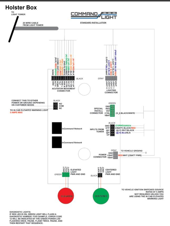
12: COMMAND LIGHT DOES NOT HAVE POWER 13: COMMUNICATION ISSUE BETWEEN THE KEYPAD AND MAIN BOARD 14: DOES NOT HAVE CONTROL OF SYSTEM (VMUX ONLY)
