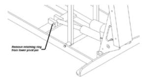
Note that the light weighs in excess of 100 pounds, use caution. Apply upward pressure on the main lift arm to remove support blocking then slowly lower the lift arm allowing the actuator shaft to extend past the lower pivot blocks.
