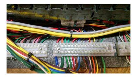
Wire the small gray 22-20 control cable to the 20 pole strip color for color. Crimp the provided  $2 \text{ Awg} / \frac{1}{4}$ " hole connectors on the black and red 2 Awg cables, red goes to the open "BAT" stud on the breaker and black goes to the  $\frac{1}{4}$ " ground stud with the lamp ground wires.
