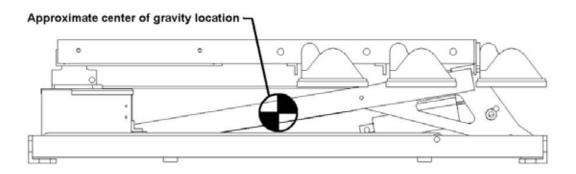
Slowly lift the *KNIGHT<sup>SLIM</sup>* and check for balanced lifting. Lower and make any necessary adjustments to the lift points.
