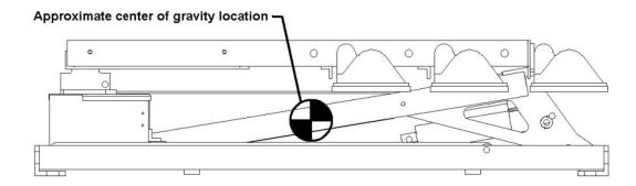
**ACAUTION** Slowly lift the *KNIGHT*<sup>SLIM</sup> and check for balanced lifting. Lower and make any necessary adjustments to the lift points.
