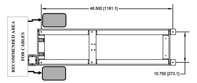
Four mounting bolt holes are required. Additional holes may be drilled in the frame ends if necessary to clear obstructions.
