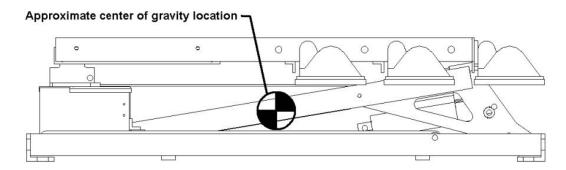
**ACAUTION** Slowly lift the *KNIGHT*<sup>2</sup> and check for balanced lifting. Lower and make any necessary adjustments to the lift points.
