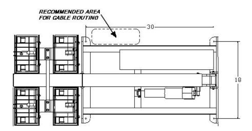
Four mounting bolts are required. Additional holes may be drilled in the frame ends if necessary to clear obstructions.
