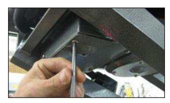
Swap the wires from the old motor to the new motor. Now the new motor can be installed.
