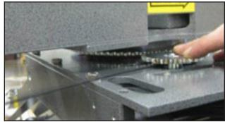
8. If not already, loosen up the four motor screws to let the motor slip for adjustment. Wrap the chain back around the sprockets bringing the ends together.
