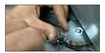
3. Using a 3/32 allen wrench, Remove the two set screws in the small sprocket. Gently pull off the small sprocket.
