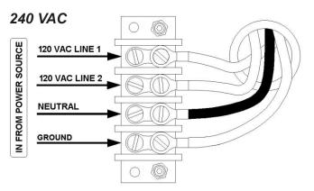
If 240 VAC operation is desired, remove the jumper wire between the red and black leads.
