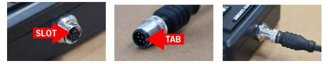
Make sure the tab on the coil cord connector lines up with the slot on the controller connector. Rotate the coil cord connector clockwise until finger tight. **DO NOT** use tools to tighten this connector.
