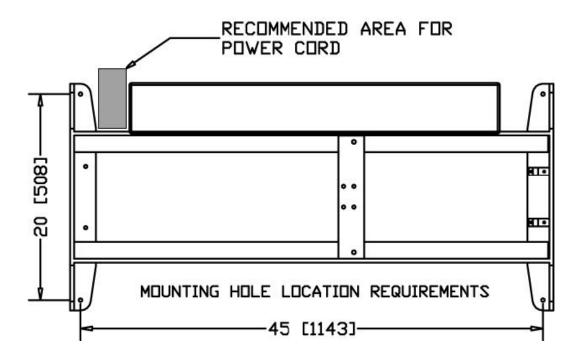
Four mounting bolt holes are required. Additional holes may be drilled in the frame ends if necessary to clear obstructions.
