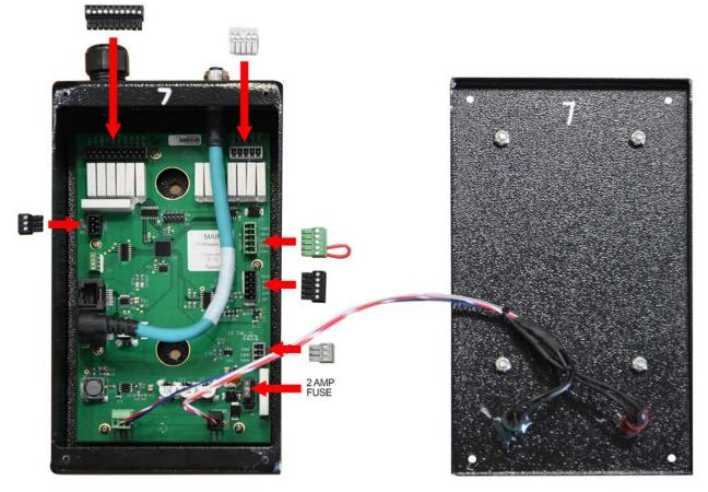
**Detaching & Attaching the Controller**
