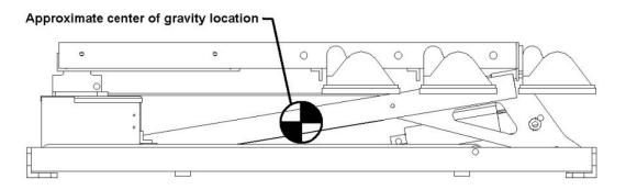
**CAUTION** Slowly lift the *KNIGHT*<sup>2</sup> and check for balanced lifting. Lower and make any necessary adjustments to the lift points.
