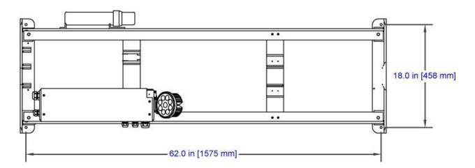
Four mounting bolts are required. Additional holes may be drilled in the frame ends if necessary to clear obstructions.
