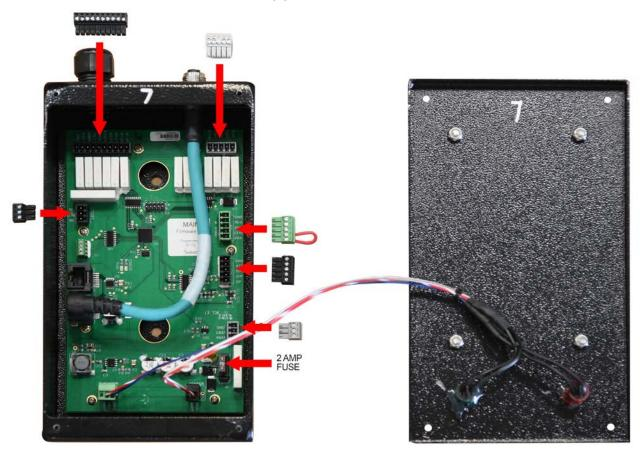
**Detaching & Attaching the Controller**
