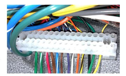
Wire the small gray 22-20 control cable to the 20 pole strip color for color. Crimp the provided 2 Awg /  $\frac{1}{4}$ " hole connectors on the black and red 2 Awg cables, red goes to the open "BAT" stud on the breaker and black goes to the  $\frac{1}{4}$ " ground stud with the lamp ground wires.
