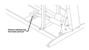
**ACAUTION** The light weighs in excess of 100 pounds, use caution. Apply upward pressure on the main lift arm to remove support blocking then slowly lower the lift arm allowing the actuator shaft to extend past the lower pivot blocks.
